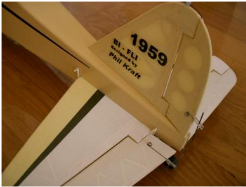
“Bi-Fli” tail showing torque rod connections to Rudder and Elevator. Designed by Phil Kraft 1959
