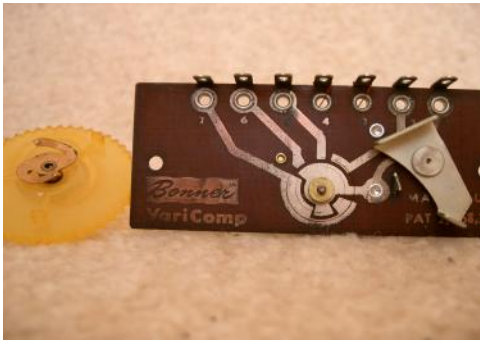
Control / output wheel removed to show its wipers at rear and the printed circuit mounting board.
